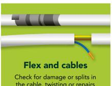
the cable, twisting or repairs with adhesive tape.
